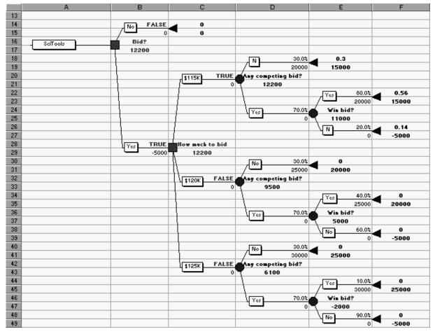
FIGURE 10.2 Result of Folding Back to Obtain Optimal Decision
